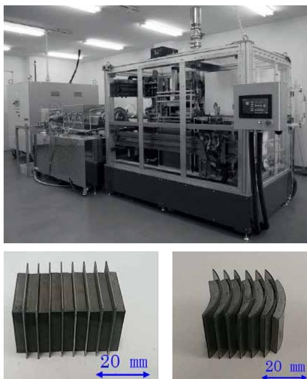
**Fig 3.66:** A New Pressless Process equipment along with the near net shaped slab and arc magnets manufactured using the technology.
