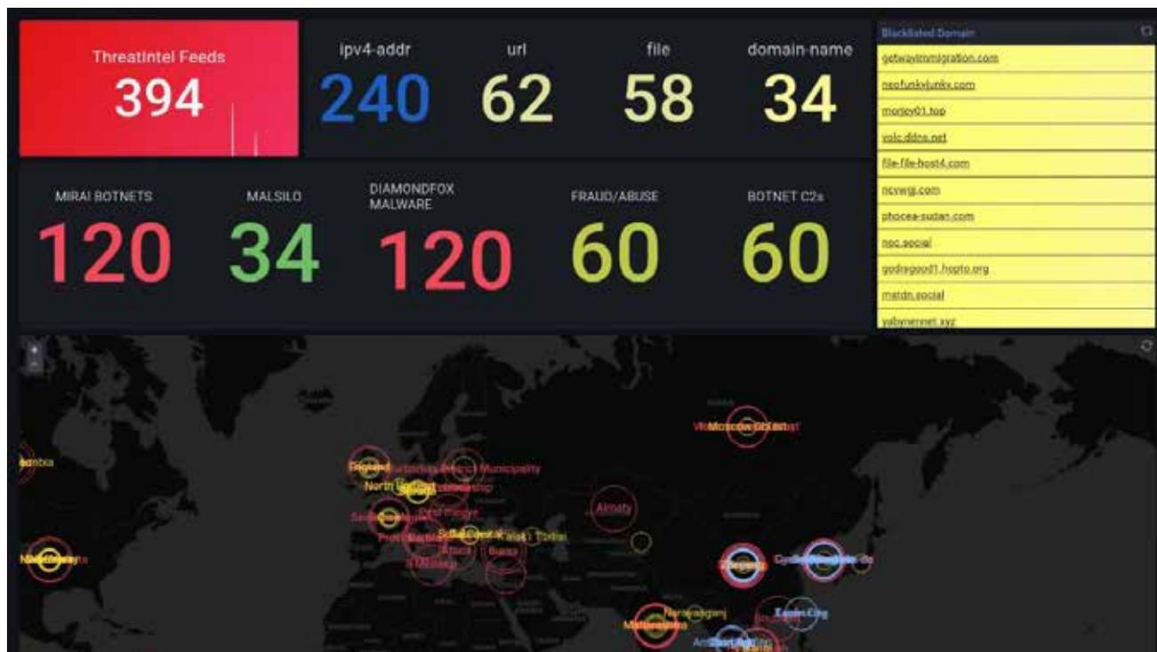
Fig 3. 63: Screen of the C3i Honeypot Dashboard Showing Collected Threat Intelligence
