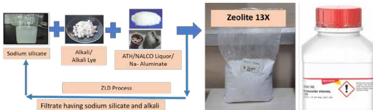
Fig 6.2: Zeolite 13X powder preparation process
