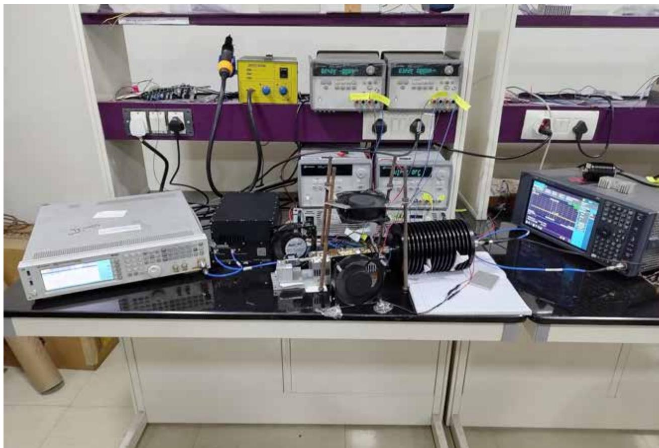
Fig 4.27: Measurement setup for Doherty power amplifier (DPA).
