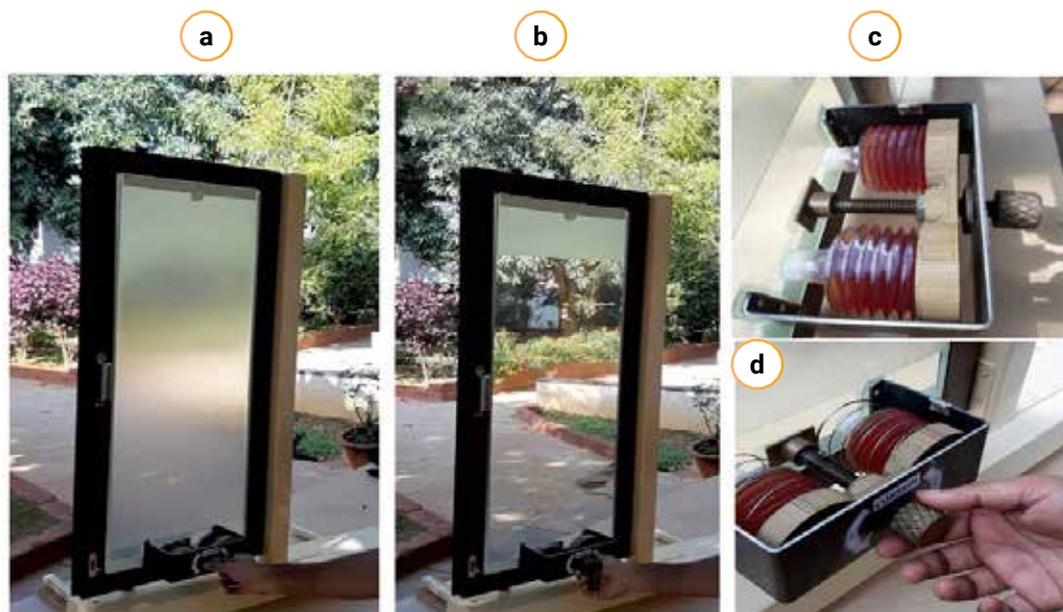
**Fig 3.81:** Shows the smart window device with bellow compression/expansion-based pumping mechanism wherein (a) is the device in the translucent state, (b) is the device in the transparent state, (c) is a close view of the pumping mechanism, and (d) provides operation of pumping mechanism with knob rotation.
