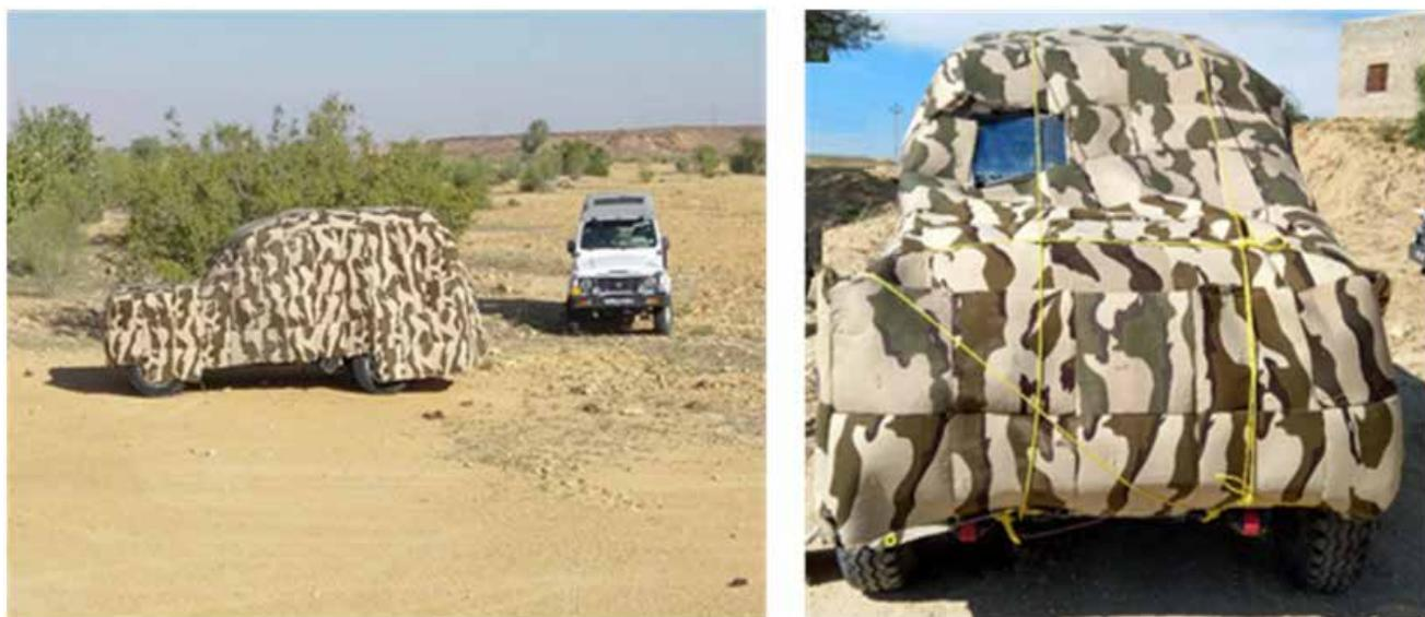
Fig 5.3: Test vehicle covered with textile-based metamaterial absorber and reference vehicle. The Vehicle window is covered with an optically transparent absorber.
