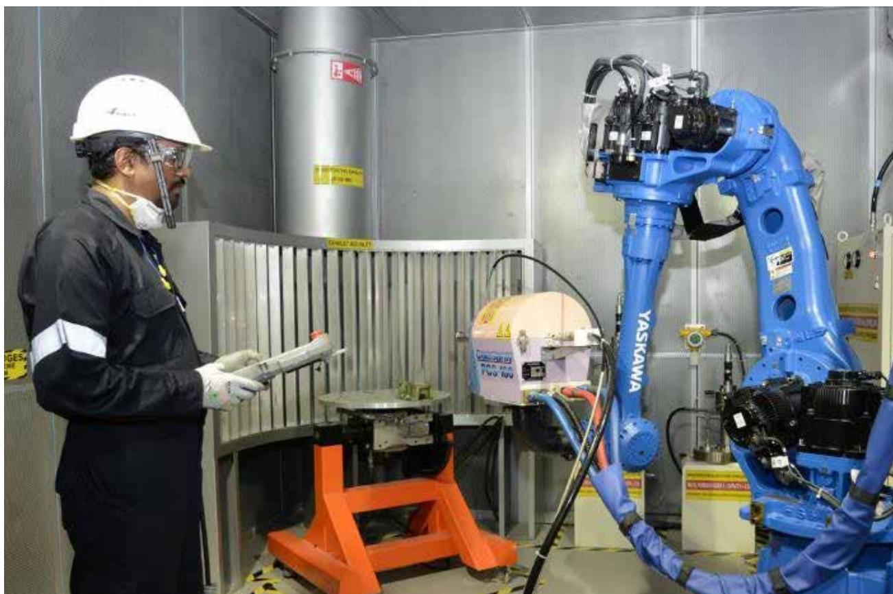
Fig 5.8: High-pressure cold spray system (IITM)
