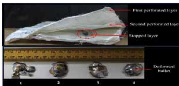
Fig. 4.29: Homogeneous SAP made from DPE tape laminates and deformed bullets
