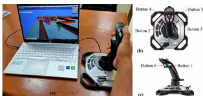
**Fig. 4.40:** VR setup with joystick and the subject performing the tasks, (b) Top view of the joystick, (c) Side view of the joystick.
