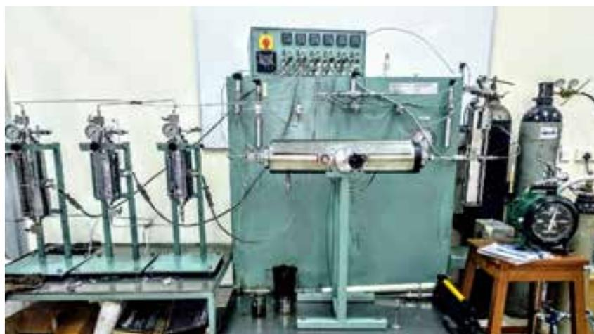
Fig. 3.7: The core flooding System.
